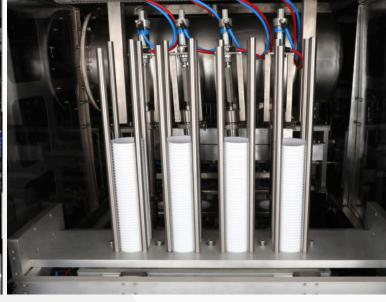
A Linear Cup Filling Sealing Machine is an automated system designed for high-speed filling and sealing of cups in a linear process, ideal for dairy, beverage, and food industries. It handles various cup sizes and materials efficiently, ensuring consistent filling accuracy and secure sealing.
